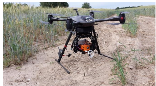
Figure 4. COSI camera mounted on the Aerialtronics Zenith octocopter
